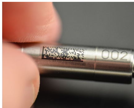
Annealing on stainless steel
